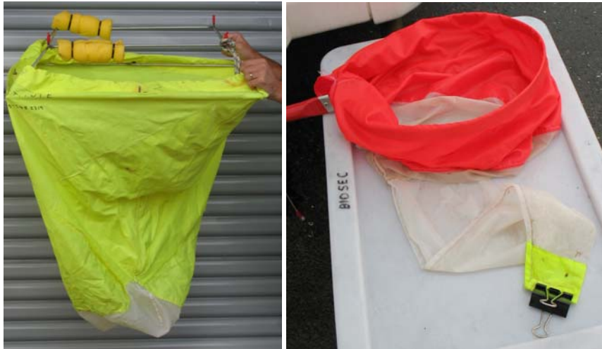
Figure 4: Diver-operated collection bags (60 \mu\text{m} mesh size) used during the defouling trials to capture defouled material not collected by the rotating brush systems.
