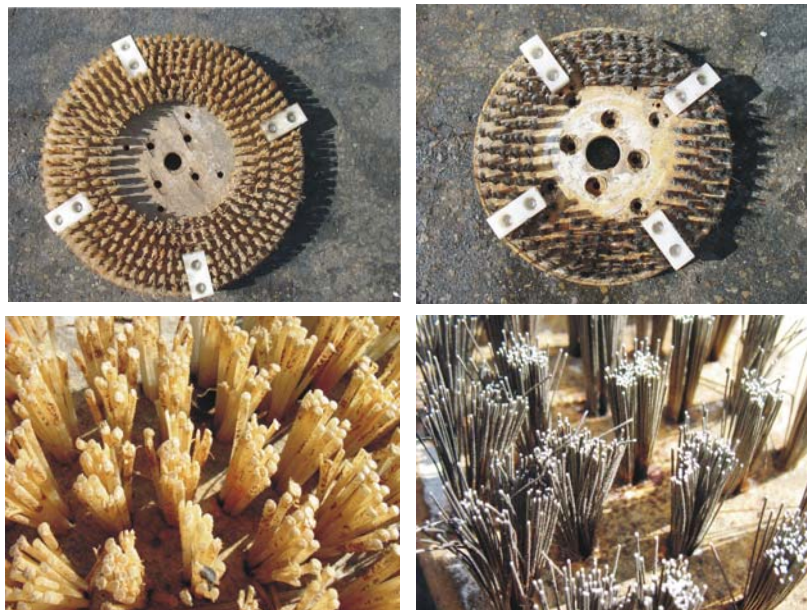
Figure 37: Examples of brush types (diameter of brush head = 360 mm) currently available to remove more persistent fouling organisms. Note: Polyethylene (left) and stainless steel (right) bristles. Higher grades (e.g. solid polyethylene blocks) are also available.
