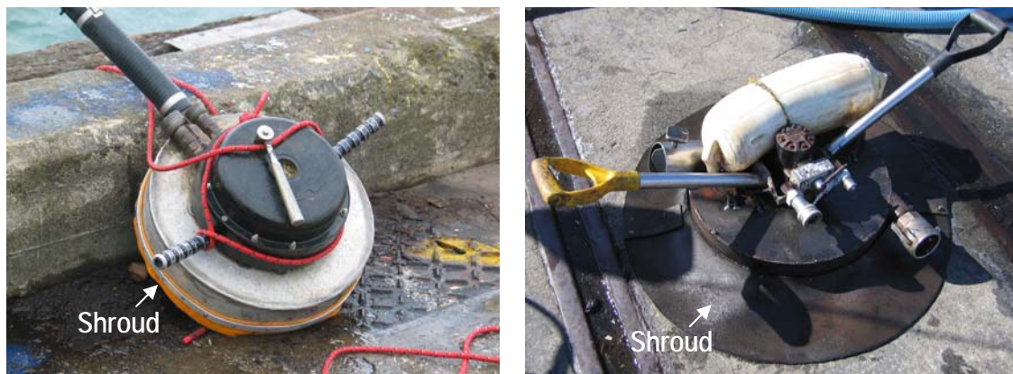
Figure 1: Rotating brush devices used in the trials. Note: Suction/collection systems are not pictured; System A (left) and System B (right).
