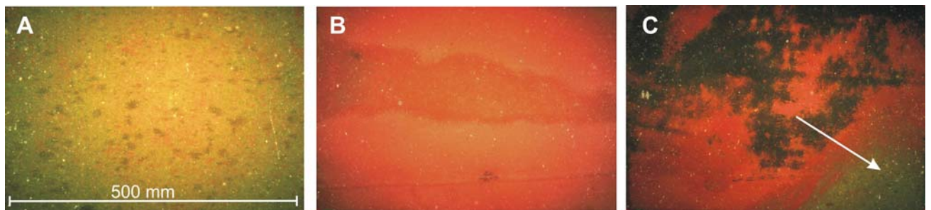
Figure 35: Representative photographs of 1m x 1m test areas on a fouled vessel. (A) before and (B) after defouling; (C) sections missed by divers.
