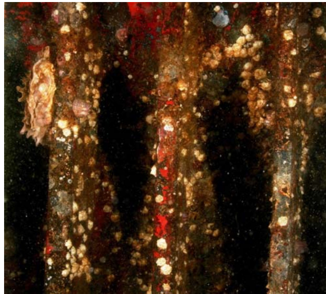
Figure 39: An example of a niche area of a vessel that would be inaccessible to rotating brush systems.
