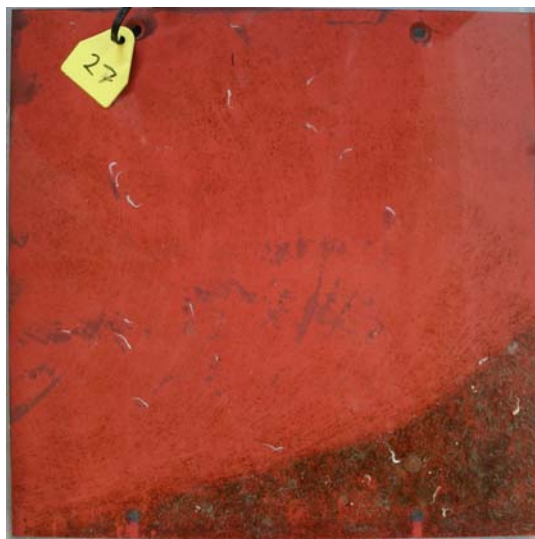
Figure 34: A photograph of a flat settlement plate following a defouling treatment. Deployment time = 3 months. The bottom-right section of the plate was 'missed' by the divers during the treatment (i.e. diver error).
