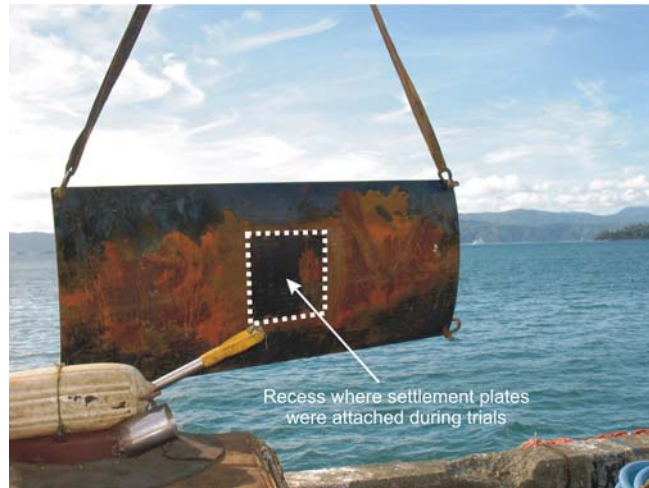
Figure 3: The metal backing plate used to replicate curved areas of a vessel hull. Note: System B is in the foreground.
