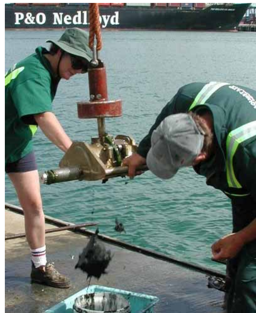
Figure 9: Shipek grab sampler: releasing benthic sample into bucket
