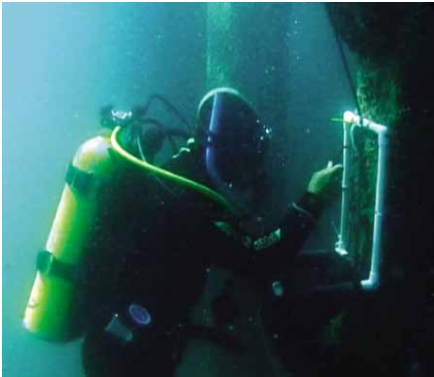
Figure 8: Diver sampling organisms on pier piles.
