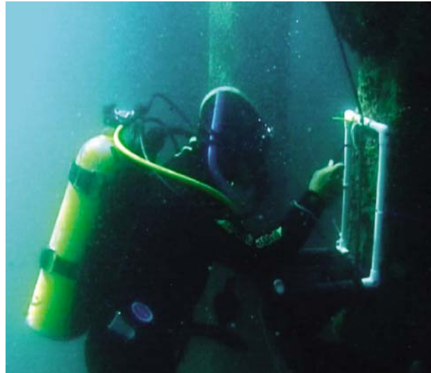
Figure 4: Diver sampling organisms on pier piles.
