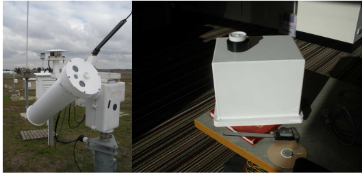
Figure 2. On the left is the ASR deployed at Melbourne Airport, and on the right the Pi-radiometer, next to a CD-ROM to provide an indication of size.
