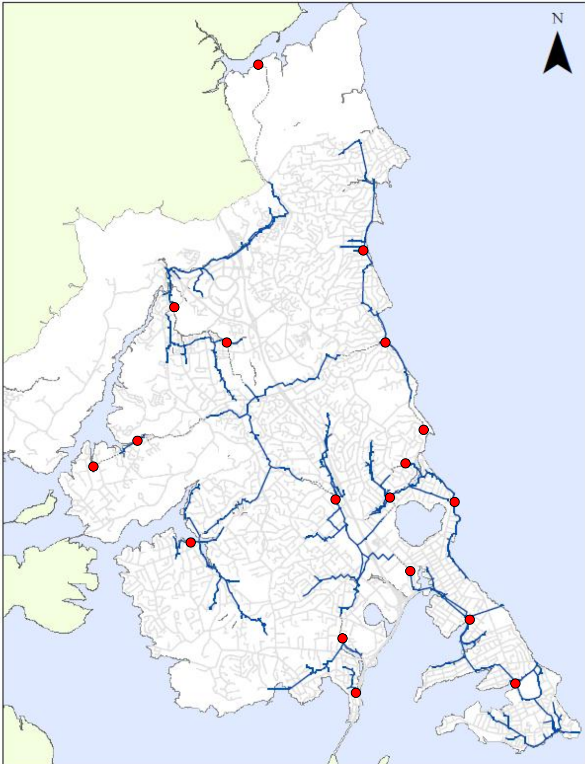
Figure 2.1: Model extent for the NSCC waste water network showing location of trunk sewers (blue lines), rising mains (grey dashed lines) and modelled pumping stations (red circles). Modified after Lockie and Brown, 2010
