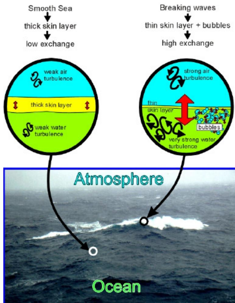
Figure 2. Physical processes at the air-sea interface.
