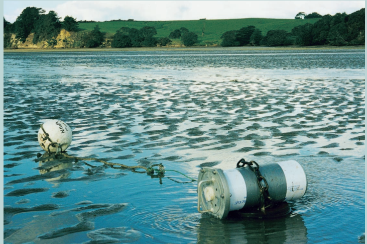
DOBIE moored in Okura Estuary (North Shore) for measuring waves on the intertidal flat.
