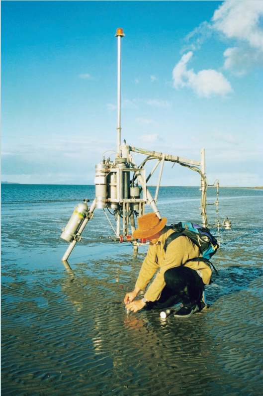
Instrumented tripod (ALICE) at Okura to measure near-bed currents, turbulence and sediment transport.
