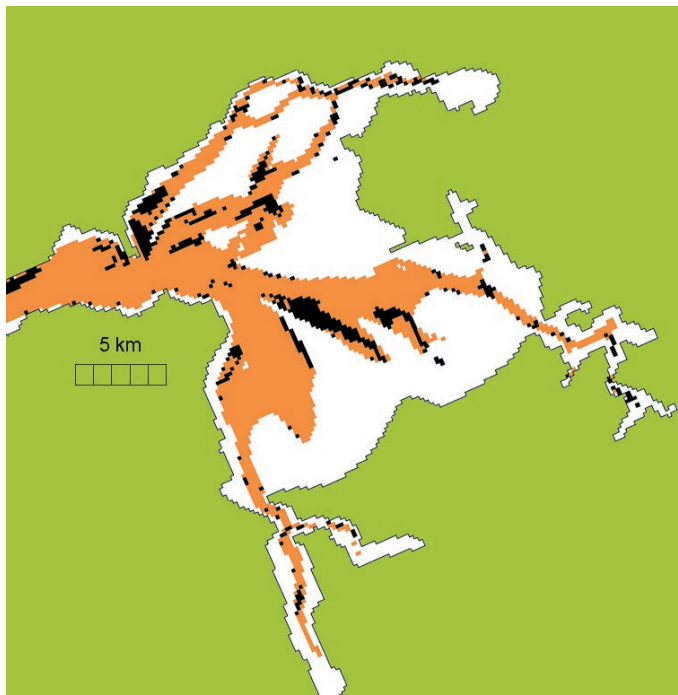
Model simulation of the tidal channels of Manukau Harbour (see Green et al. 2000). Brown indicates ebb-tide dominance and black indicates flood-tide dominance. White areas are intertidal sandbanks.
