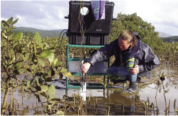
A NIWA technician measures microprofiles of dissolved oxygen, hydrogen sulphide, and pH in mangrove mud using electrochemical microsensors.
