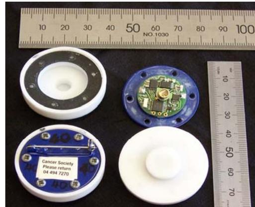
**Figure 1.** Electronic UV dosimeter badges + PTFE diffuser cap.
