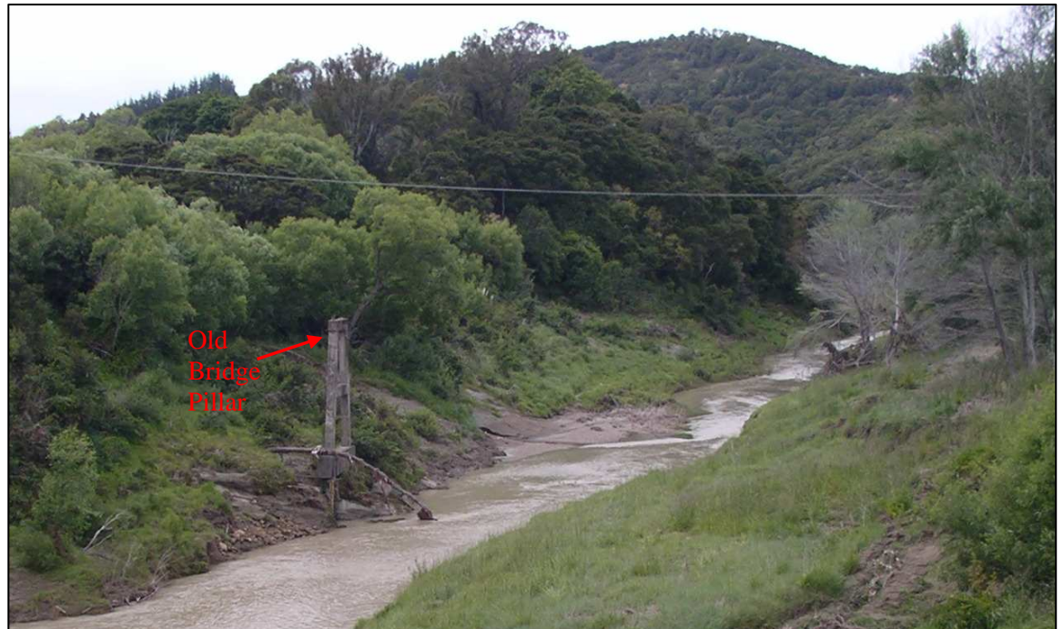
Figure 7: The flood gauge on the Hikowai branch of the Uawa River (Willow Flat) provides a reminder of the power of the Uawa River in flood. When the river stage reaches the top of the old bridge pillar shown (12 m) the council activates its evacuation plan for the lower flats; during Cyclone Bola the stage reached 3 m above the pillar (15 m). Photo: H.K. McMillan
