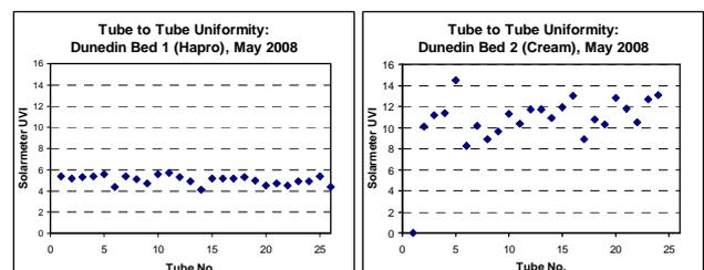
**Figure 2.** Tube to tube uniformity in two sunbeds
