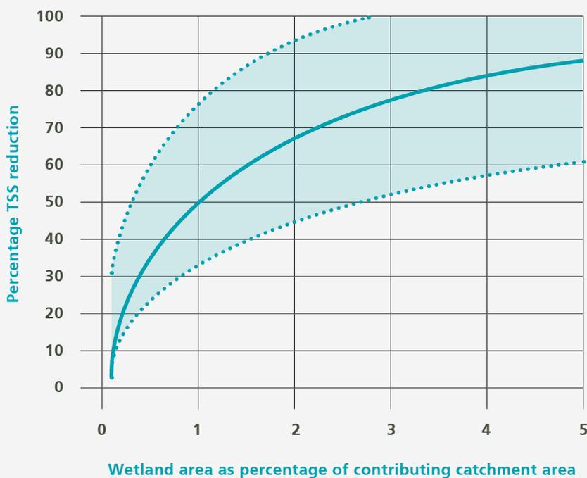
**Figure 1:** Long-term median annual performance expectations for reduction of Total Suspended Solids (TSS). Performance is for appropriately constructed wetlands receiving surface runoff and drainage from pastoral farmland in New Zealand. Not applicable to areas with clay soils ( $\geq 35\%$  clay content) or catchment rainfall outside NZ norms as noted in the text. Solid line shows expected median. Shaded area shows expected inter-annual and inter-site range of performance.
