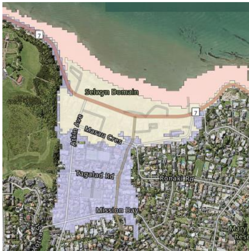
Figure 1-1: Example of the extreme coastal flood maps. Mission Bay, Auckland. Pink = present-day 1% AEP coastal flood exposure. Yellow = +1 m RSLR. Blue = +2 m RSLR.
