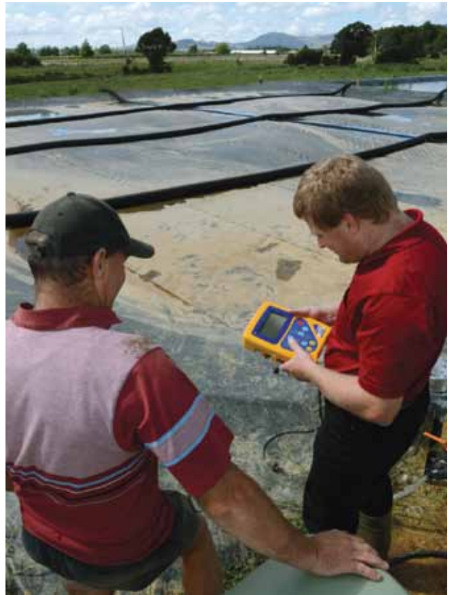
Farmer Neville Barr (L) and NIWA resource engineer Stephan Heubeck use a gas analyser to measure levels of methane, carbon dioxide, hydrogen sulphide and oxygen from the covered anaerobic digester pond beyond. (Dave Allen)
