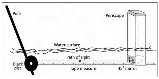
Figure 5.8: Schematic of black disc method of water clarity measurement. *Illustration: Rob Davies-Colley*
