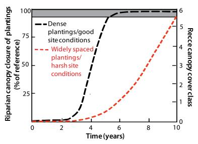
Figure 5.42: Hypothetical rates of canopy closure of riparian plantings (on banks and not over the stream) over a 10-year period (subject to monitoring, pest control, and other post-planting maintenance). Estimated Recce cover class for a tier of  $0.3-2~\mathrm{m}$ .
