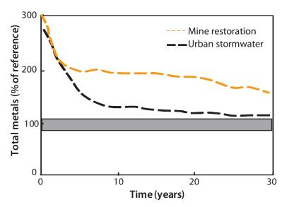
Figure 5.30: Hypothetical response curves for total metal concentrations under two restoration scenarios: 1) treatment of inflow stormwater to an urban stream with detention ponds and constructed wetlands, and 2) restoration of a forested stream below an abandoned mine that still has sources of heavy metal contamination.
