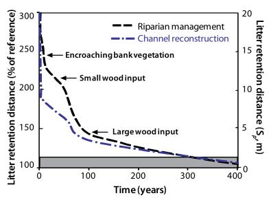
Figure 5.15: Hypothetical retention distance of leaf litter inputs after riparian management and channel reconstruction, based on differences between  $S_p$  of pasture and forest stream reaches in straightened and natural channels (James & Henderson 2005, Quinn et al. 2007).
