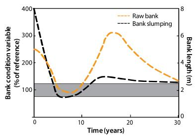
Figure 5.3: Hypothetical timescales for the length of stream bank affected by bank slumping or raw banks following riparian management (fencing and planting) of a pasture stream reach (100 m long).
