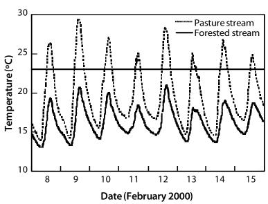
Figure 5.20: Stream water temperature recorded in a poorly shaded pasture stream and nearby forested reference stream in the Gisborne District (RDC unpublished data). The Cox-Rutherford index calculated during summer (February) low flow conditions is shown as a bar at 23 °C. This temperature index can be compared with constant temperature criteria for thermal tolerance.
