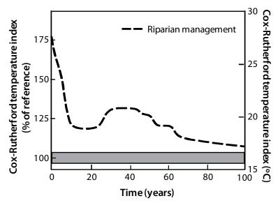
Figure 5.21: Recovery of thermal regime of a 3.3 m wide stream in the central North Island, planted with native trees that progressively re-shade the channel (model predictions from Davies-Colley et al. 2009). The Cox-Rutherford temperature index value of a reference stream (about 16°C) is not approached until the climax forest grows to its full height at about 200 years (not shown).
