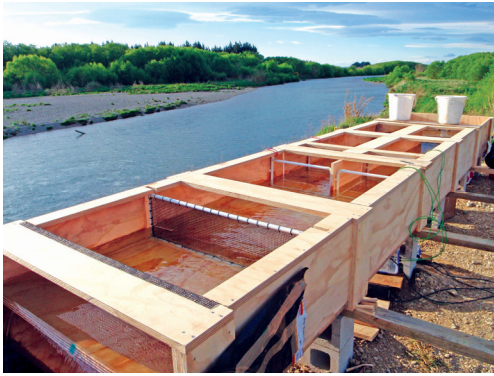
Figure 1: Choice-chamber flume to test kanakana attraction.
