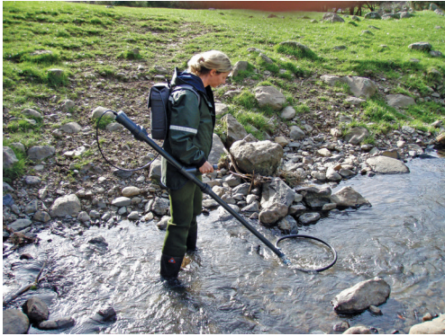
Figure 6: Hand-held PIT detector for monitoring tagged kanakana.
