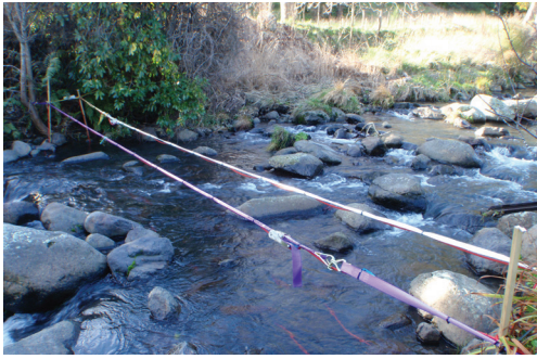
PIT antenna to monitor movements of tagged kanakana.
