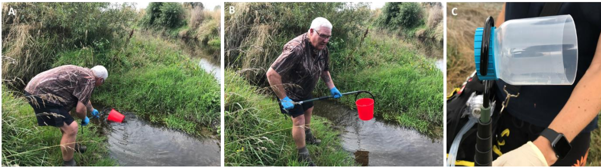
Figure 5-1: Water collection using a decoy retrieval stick. A & B, collecting approximately 5 litres of water for processing. C, use of a pottle or smaller container is also possible for easier retrieval of a water sample from the thalweg (i.e., the deepest or main flow of the stream).
