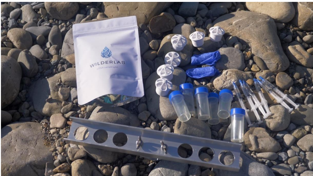
Figure 8-1: Wilderlab passive sampler kit equipment including two pairs of gloves, six filter pods, syringes and pottles and one manifold mount. Images sourced from https://wilderlab.co.nz .
