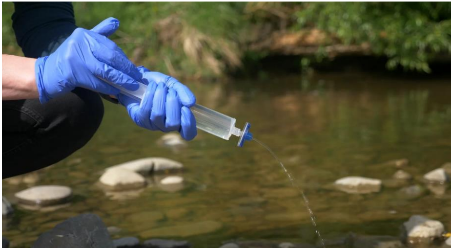
Figure 7-2: Active eDNA sampling using the Wilderlab barrel syringe and filter. Image sourced from https://wilderlab.co.nz .
