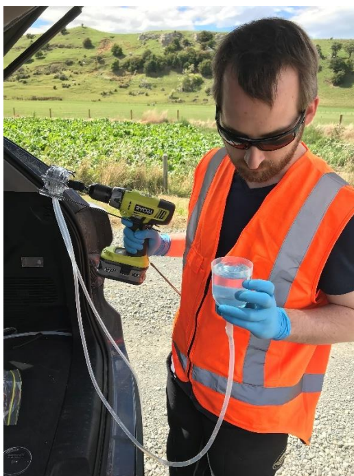
Figure 6-1: Peristaltic pump head fixed to an 18 volt battery powered drill to actively pump water through a glass microfibre filter.
