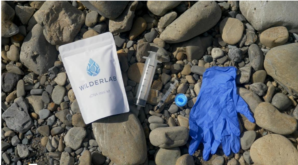
Figure 7-1: Wilderlab syringe mini kit equipment, including one pair of gloves, one large and one small syringe and one filter. Image sourced from https://wilderlab.co.nz .
