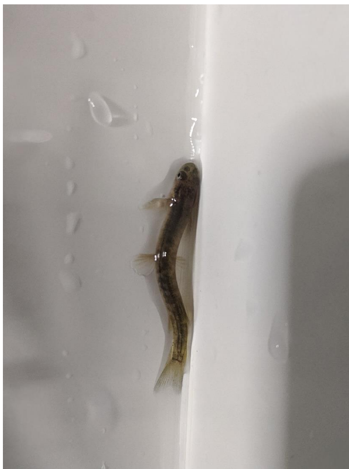
Figure 7-15: Kōaro climbing a smooth HDPE ramp in the laboratory. Photo credit: Eleanor Gee.
