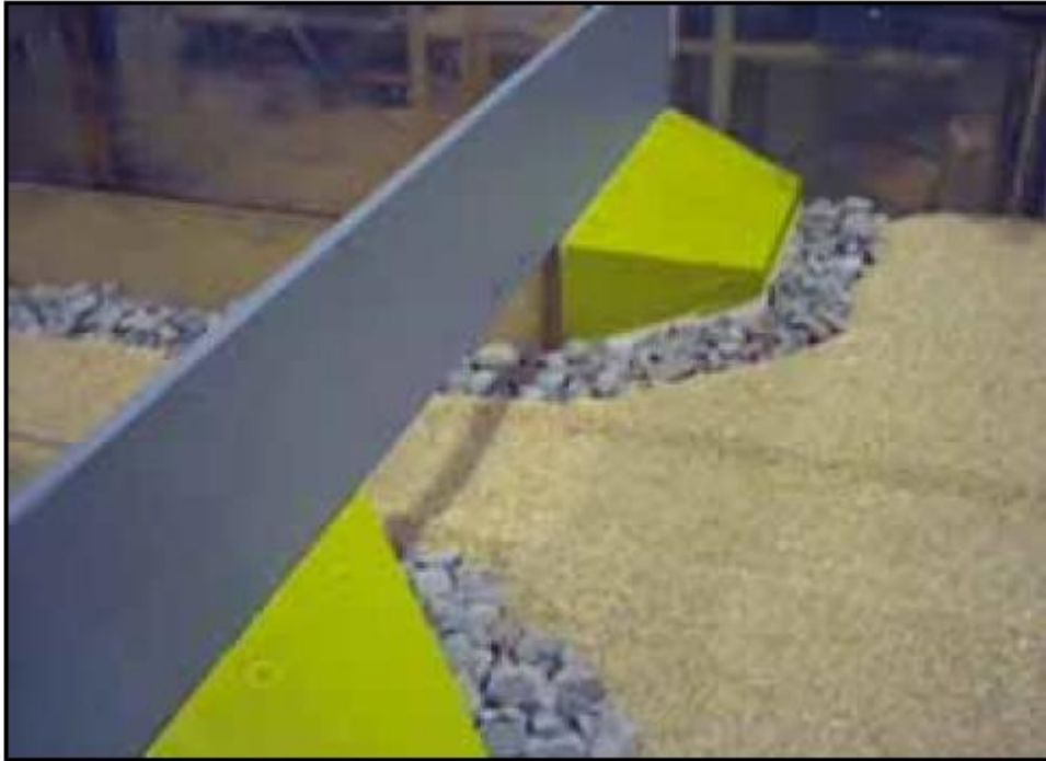
Figure 4-12: Rip-rap protection at a bottomless culvert with the MDSHA Standard Plan. Source: Kerenyi and Pagan-Ortiz (2007)
