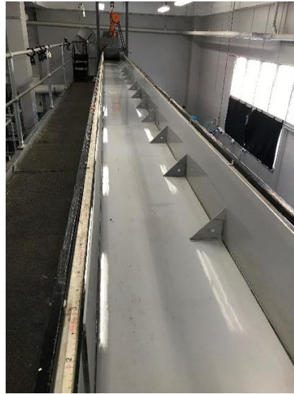
Figure J-5: Example of corner baffles. Photo credit: Craig Franklin & Rebecca Cramp, University of Queensland.
