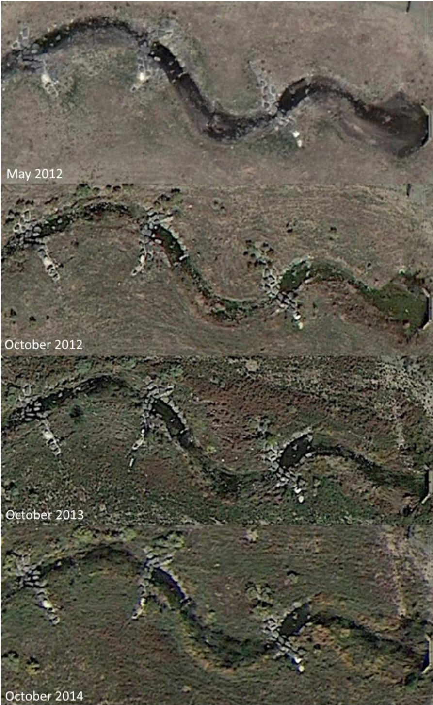
Figure G-4: Vegetation growth as part of soil rip-rap over four years following construction of a stream through a stabilised toxic waste site.
