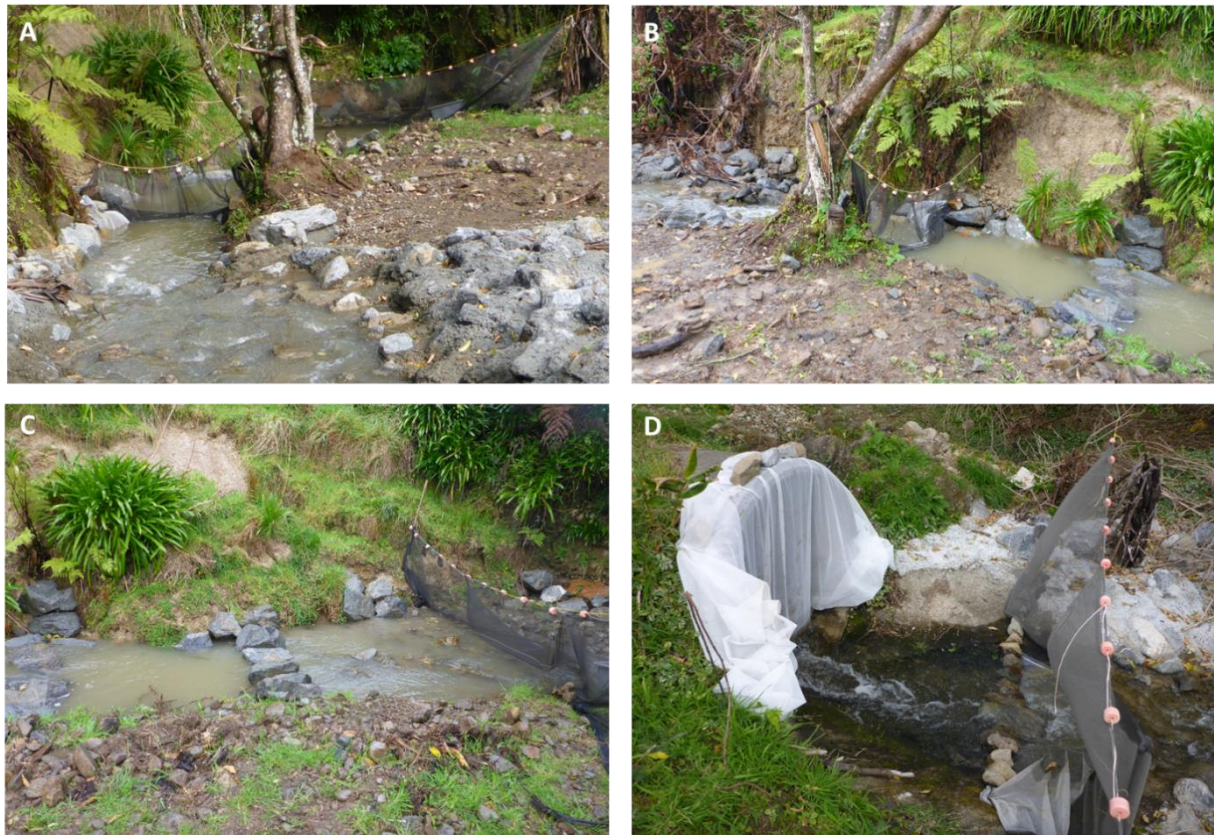
Figure 7-3: Downstream barricades installed in Kara Stream during the inanga passage trial. A - C Barrier nets deployed during the rock-ramp trial. D, Barrier nets deployed for testing inanga passage through the culvert independently of the rock-ramp.
