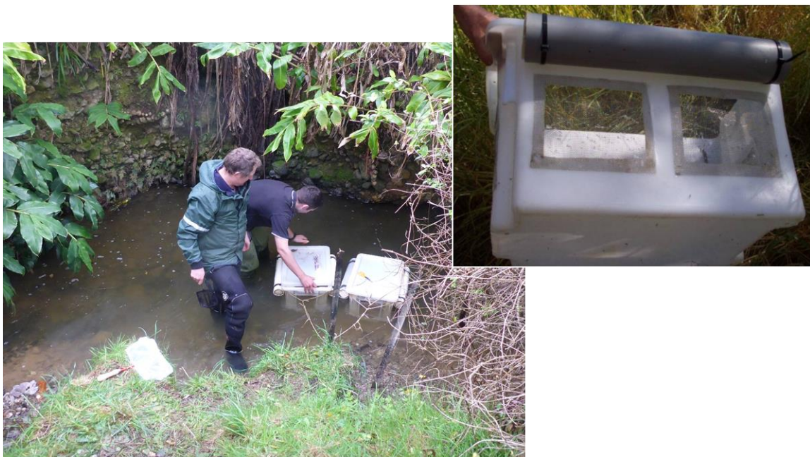
Figure 7-1: Live-bins deployed in Kara Stream to maintain inanga for fish passage trials. Inset shows close up of live-bin.
