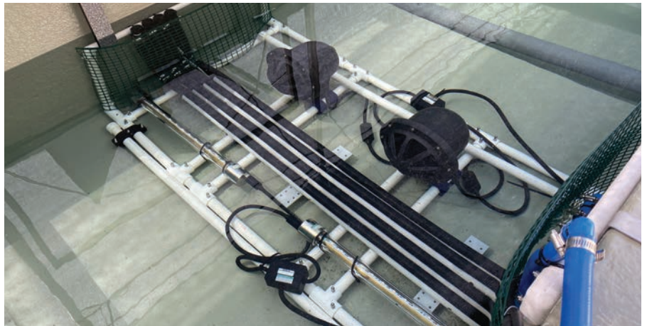
Figure 1. BAFF set up in the trial flume at Ruakura. From back of frame: the two speakers that produce the cyclic sound, the four lines of bubble tubing in the centre and two strobe lights at the front.
