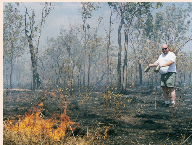
Murray McEachern (University of California, Irvine) collecting air samples for trace gas analysis from a scrub fire near Katherine, Northern Territory, Australia. The same kind of evacuated 2-litre canisters are used to collect air samples from research aircraft.
