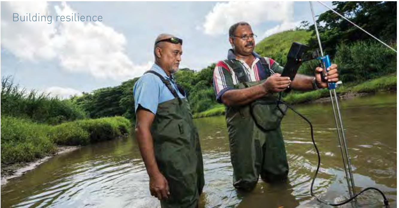
Hydrology technicians Iosefo Erenio ( left ) and Tomasi Naborisi from Fiji Meteorological Service operate new ADV (Area Depth Velocity) equipment recently supplied by NIWA to gauge river flow in the upper Nadi River catchment. Training in the use of the equipment was also carried out by NIWA. Information gathered will be used to assist in the provision of advanced flood warning to residents in low-lying areas of the Nadi Basin. [ Dave Allen ]
