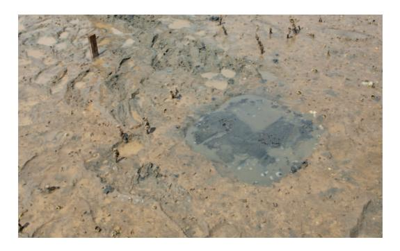
Cover the plate with the sediment that you originally dug from the hole and fill to the same level as the surrounding sediment.
