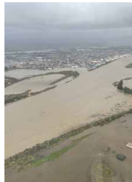
NIWA recorded a flow of 7,640 cubic metres per second for the Buller River during the July 2021 flood – the highest of any New Zealand river since 1926, and 17 times its mean flow of 454 cumecs. [West Coast Regional Council]
