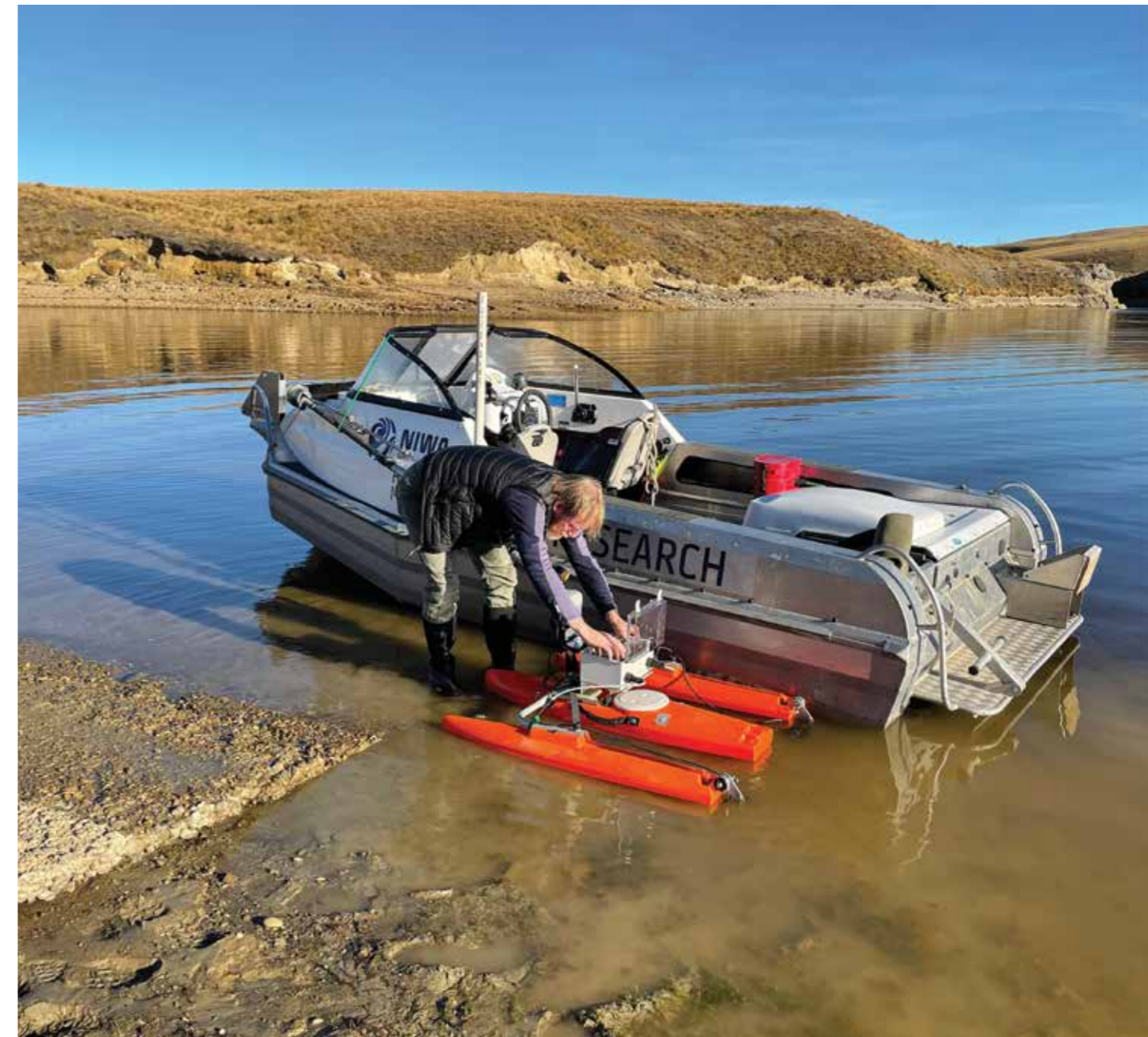
Hydrodynamics and GIS Technician Jo Bind setting up a small autonomous survey boat on Lake Onslow. [Andrew Willsman]
