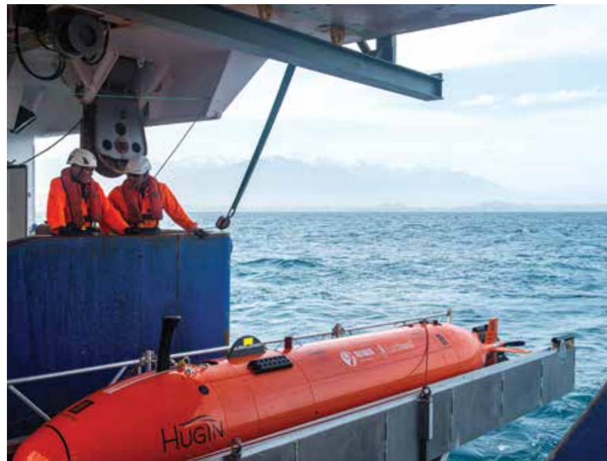
Named after the Norse Goddess of the Sea, Rán , is a 6.5m autonomous underwater vehicle deployed from Tangaroa , named after the Māori God of the Sea, to collect information on how much the Kaikōura Canyon had changed since the 2016 earthquake. [Lana Young]
