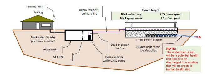
Drawing D6.1. Pump dose loading to a sand filter trench with under-drain
