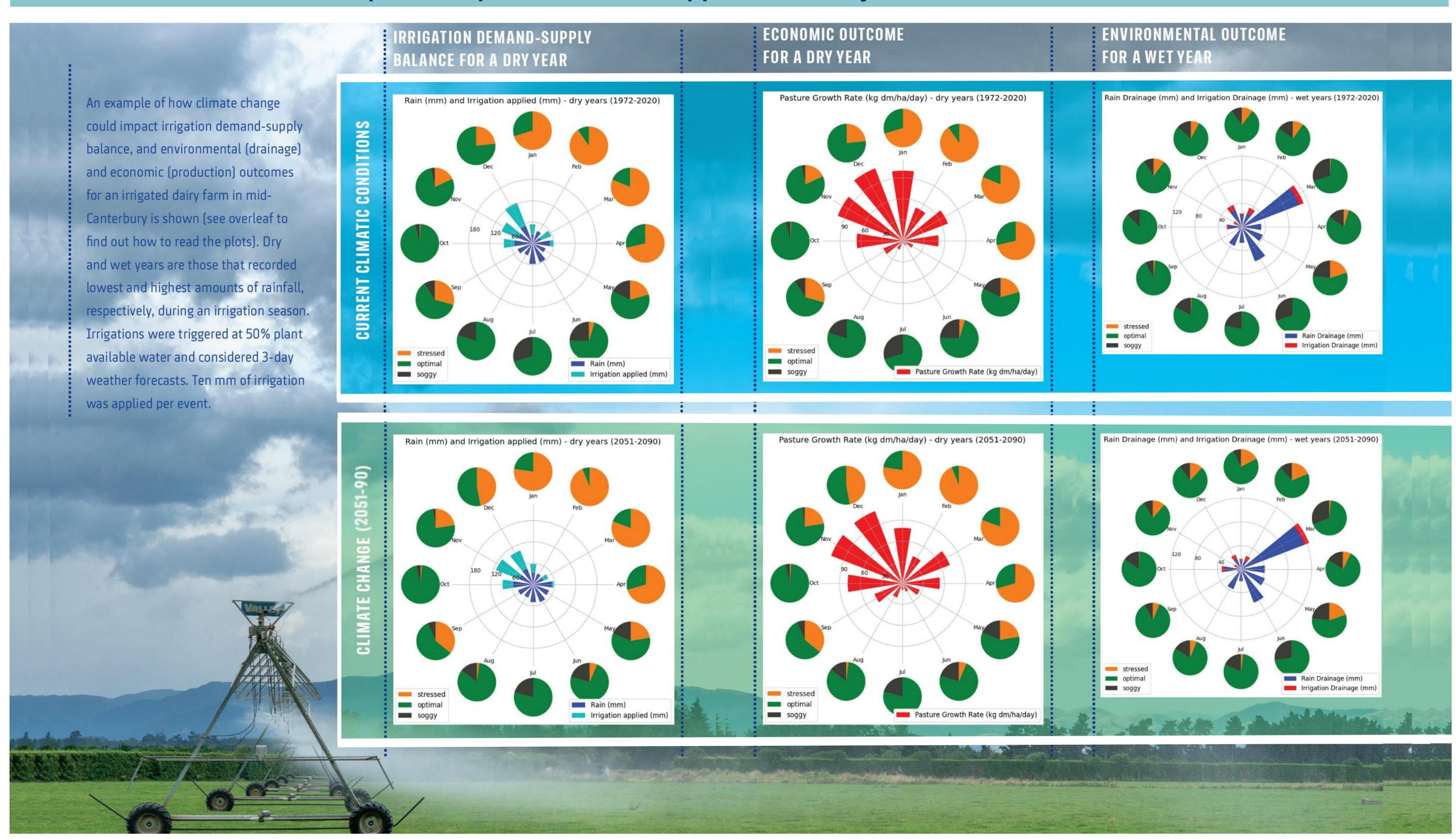
IrriSET quantifies the challenges to irrigation demand, availability and security under current and climate change for a range of irrigation scheduling practices, such as supply-based just-in-case, demand-based just-in-time, and supply and weather-forecast based justified.
