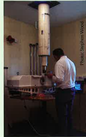
Calibrating the Dobson spectrophotometer in the new building.
