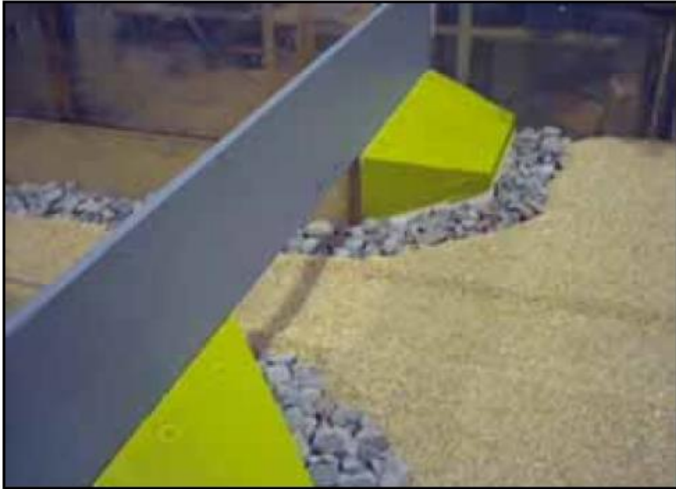
Figure 4-12: Rip-rap protection at a bottomless culvert with the MDSA Standard Plan. Source: Kerenyi and Pagan-Ortiz (2007)
