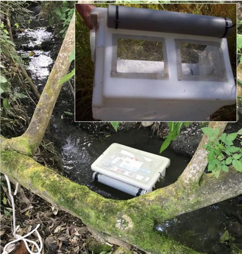
Figure 8-9: Live-bin deployed to maintain īnanga for fish passage trials. Inset shows close up of live-bin.
