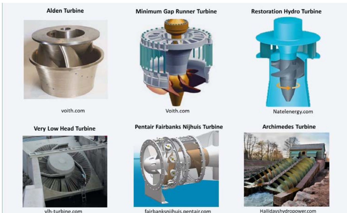
Figure 7-28: Examples of Fish friendly turbines currently used and in development internationally.
