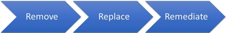
Figure 5-1: Planning for barrier remediation should follow the hierarchy of mitigation. The most effective way of restoring river connectivity is to remove the structure. If this is not possible, the next best option is to replace the existing structure with a better design that provides effective fish passage. The final option is to apply remediation to mitigate the impact of the structure on fish passage.
