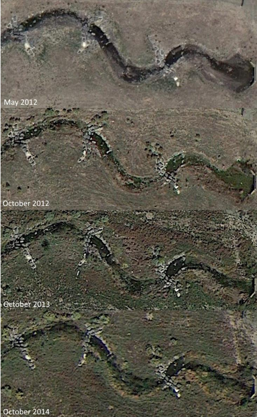
Figure G-4: Vegetation growth as part of soil rip-riprap over four years following construction of a stream through a stabilised toxic waste site.
