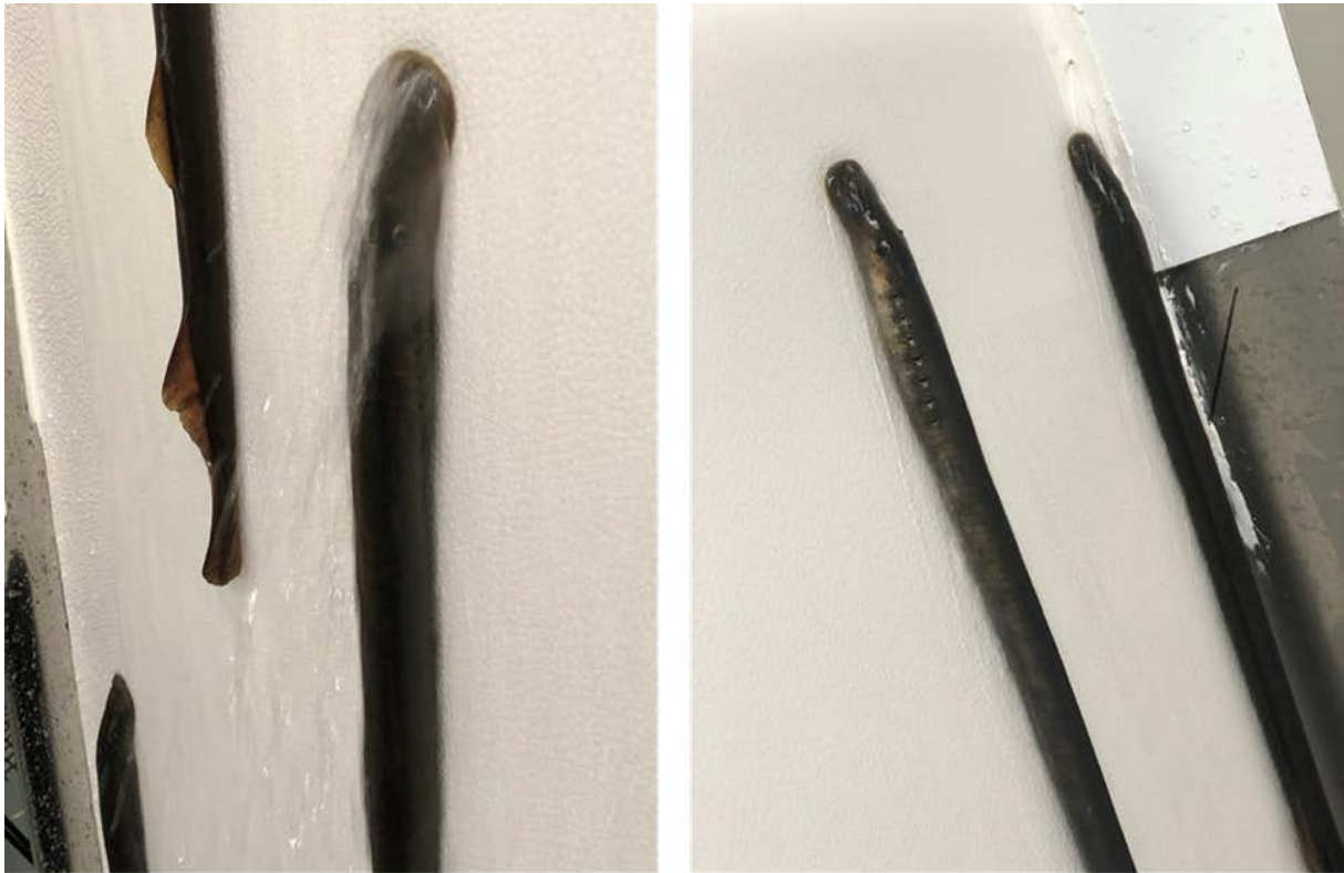
Figure 7-13: Lamprey climbing the textured HDPE ramp in the laboratory. Photo credit: Cindy Baker.
