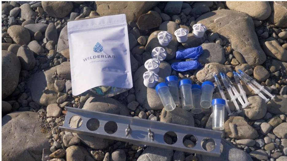
**Figure 8-1: Wilderlab passive sampler kit equipment including two pairs of gloves, six filter pods, syringes and pottles and one manifold mount.** Images sourced from <https://wilderlab.co.nz>.
