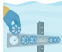
Put on a pair of gloves from the kit, and carefully push each filter pod (up to 6 can be used) into place with the leaf guard facing upstream. Ensure a tight and secure fit.
