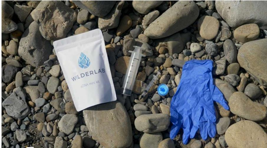
**Figure 7-1: Wilderlab syringe mini kit equipment, including one pair of gloves, one large and one small syringe and one filter.** Image sourced from Wilderlab.co.nz.
