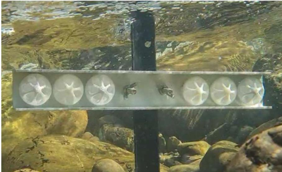
**Figure 8-2: Deployed Wilderlab passive sampler manifold attached to waratah taken within a stream.**
