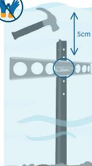
Hammer your waratah into the stream bed, in an area of moderate to high flow. Attach the passive sampler manifold to the waratah using the provided U-bolt and nuts with the edged section of the manifold facing upstream. Ensure the top of the manifold is approximately 5cm below the stream surface. Leave the manifold for approx. 5 minutes prior to inserting the filter pods to reduce the risk of cross contamination between sampling events and sites.
