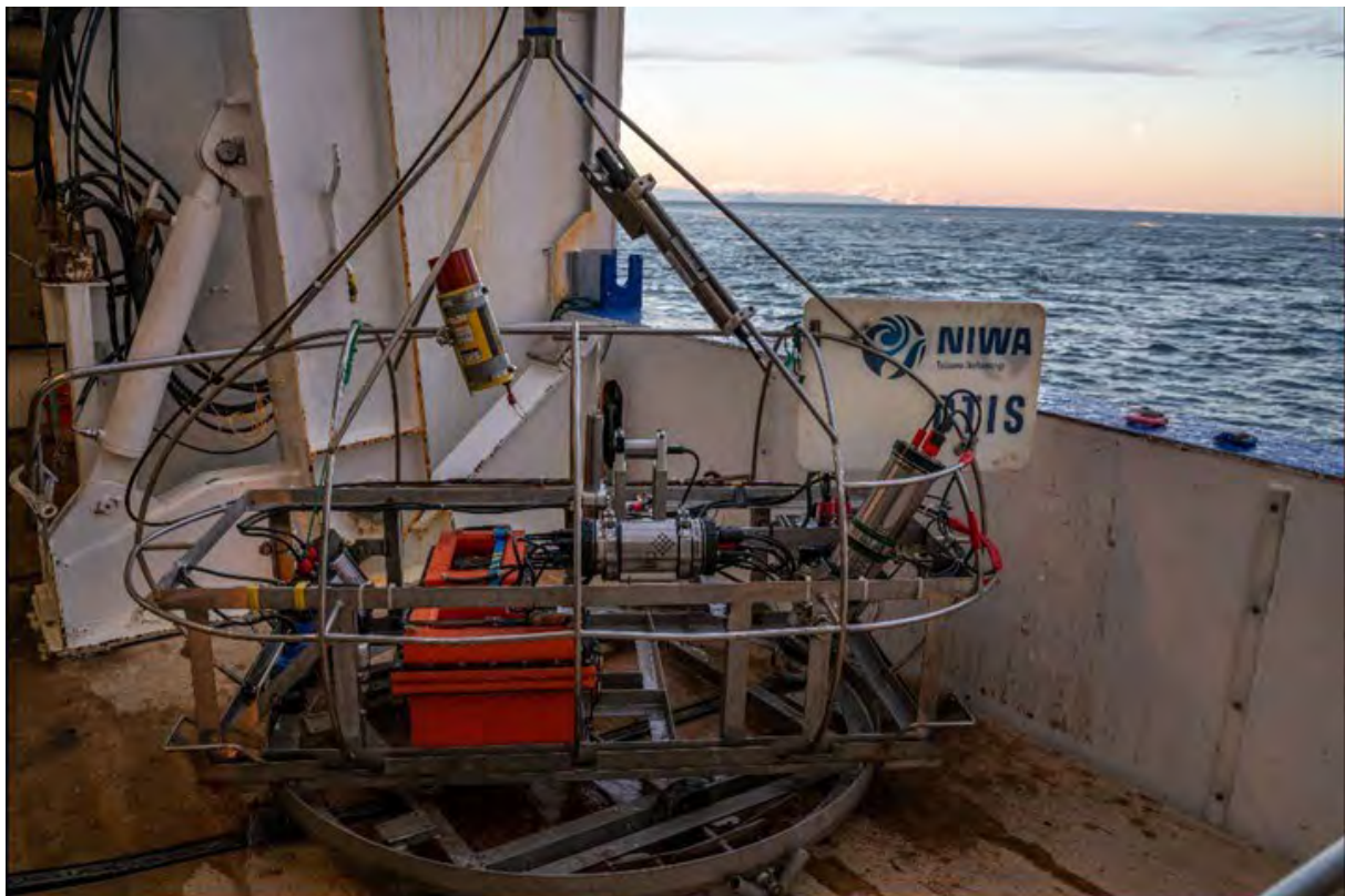
Figure 8: NIWA's towed underwater camera system, Deep Towed Imaging System (DTIS).
