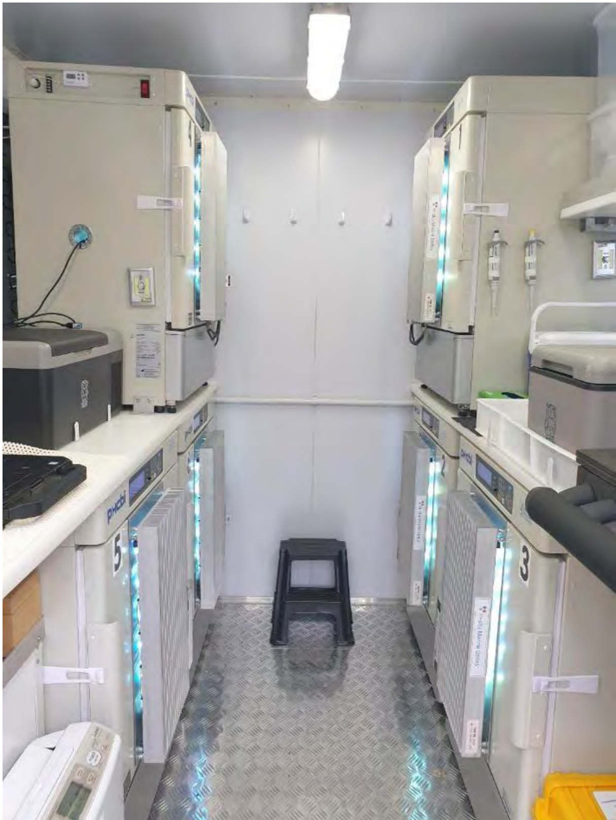
Figure 39: Simulating In-Situ (SIS) incubators. Primary productivity, grazing and bacterial production experiments were carried out in six temperature-controlled incubators with spectrally tuneable irradiance light sources (SIMs) retrofitted to incubator door windows. Incubator light intensity varying with solar irradiance across the day and spectra were tuned to collection depths using a radiative transfer model. (HydroLight/EcoLight).
