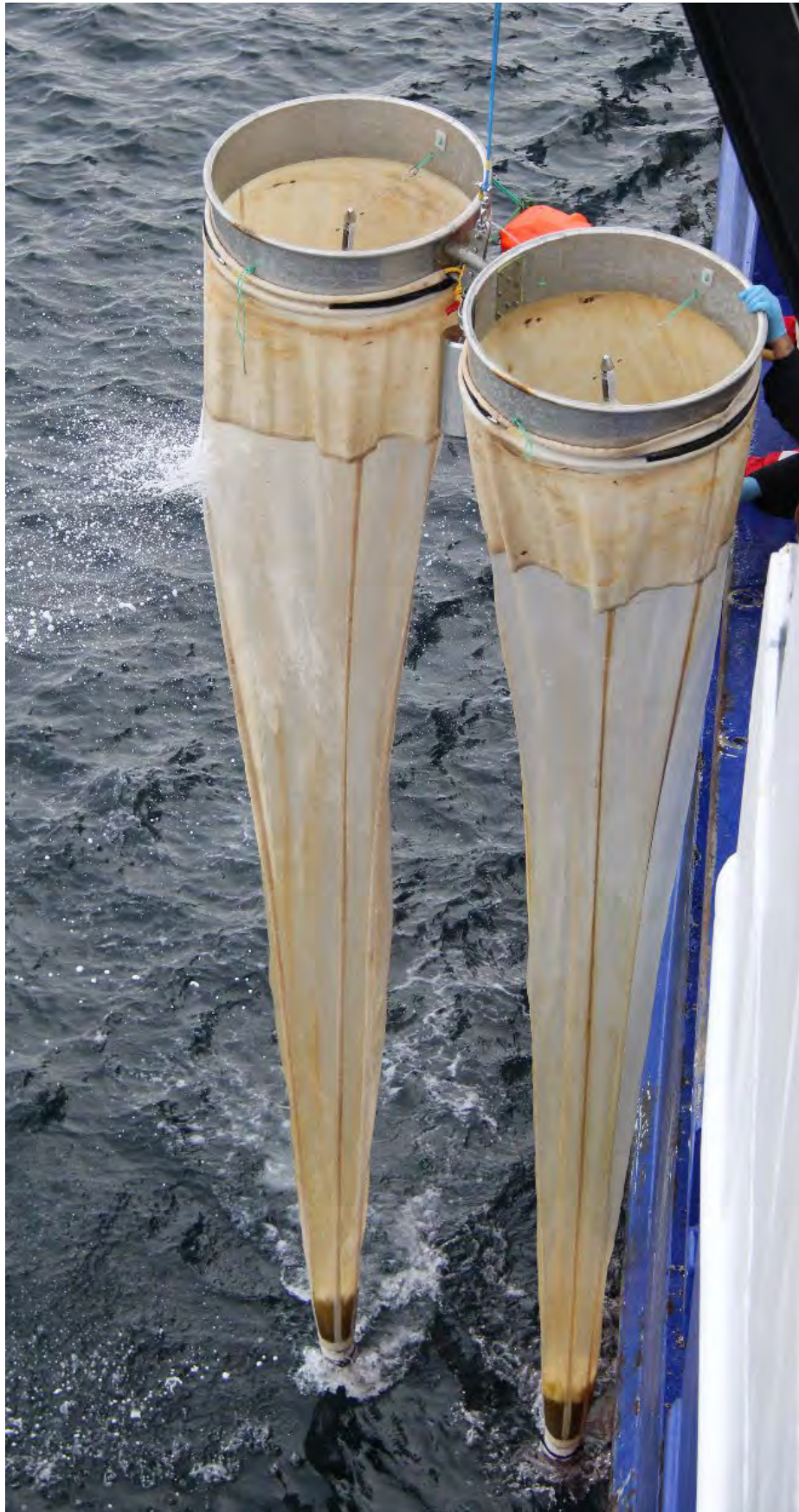
Figure 15: The Bongo net with contents being hosed down into the cod-ends over the side in the cutaway. (Photo: Gus van Wyk).
