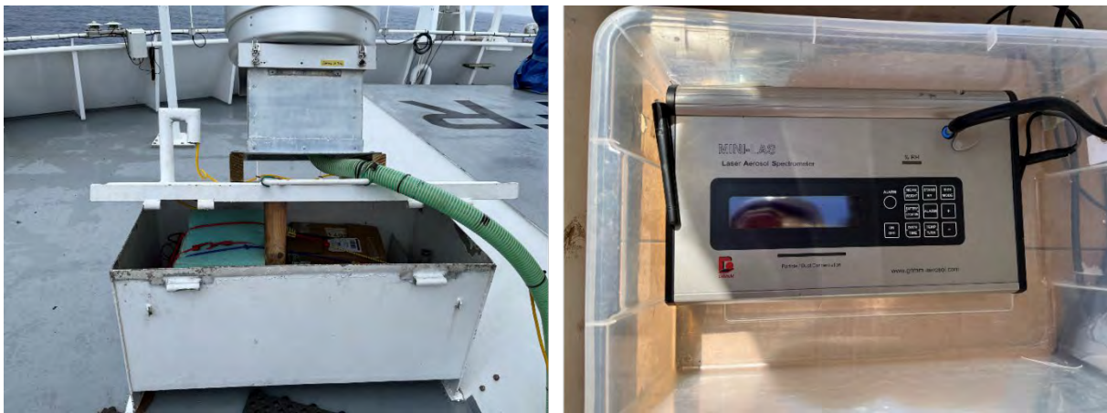
Figure 28: The Mini Laser Aerosol Spectrometer located within a metal box beneath the high-volume aerosol sampler.
