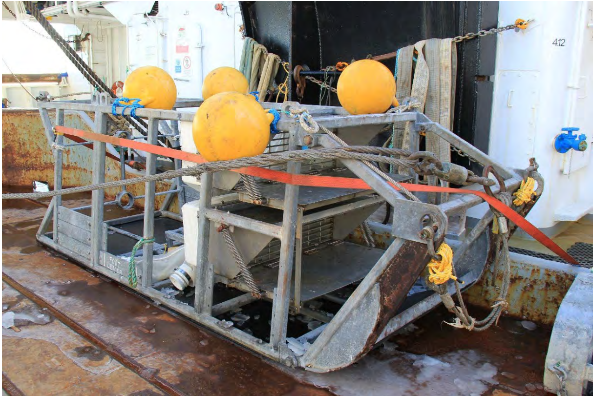
Figure 12: Brenke Sled tied down on the trawl deck.
