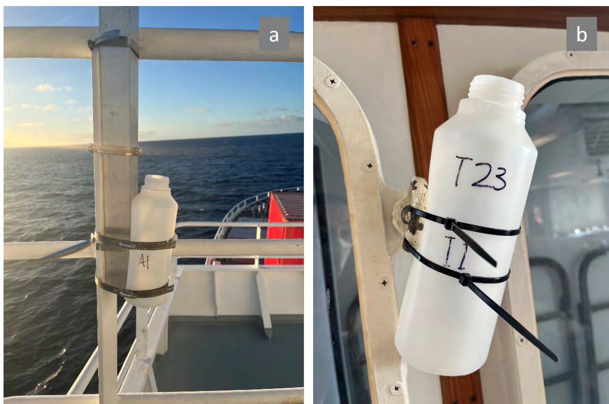
Figure 62: Microplastics bottles installed. a) portside on the railing underneath the bridge, and, b) the corner of the mess.
