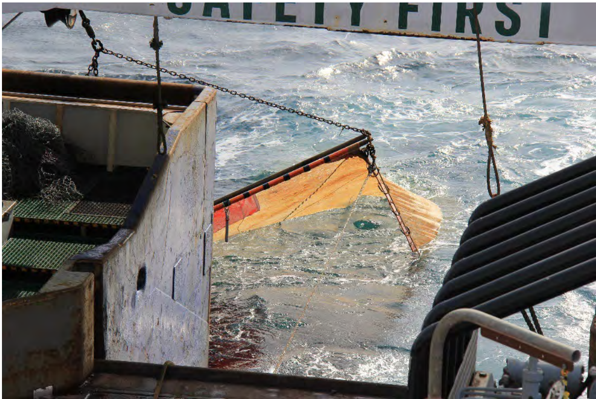
Figure 18: Deployment of the RMT using Gilson and master-pull winch. (Photo: Gus van Wyk).
