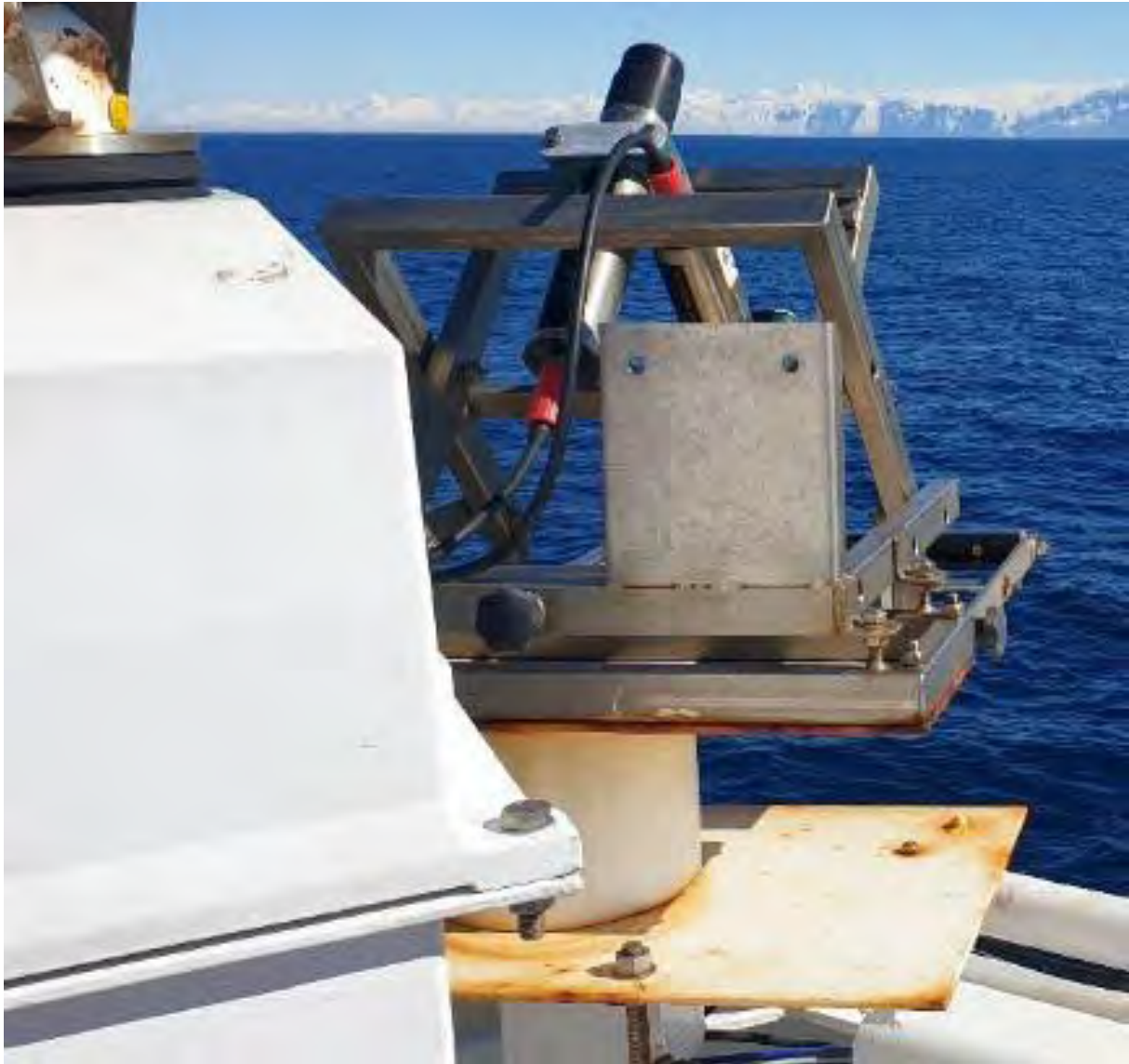
Figure 23: Sky and sea surface viewing hyperspectral radiance sensors on the port forward rail of the monkey island. Ideal sea surface viewing conditions are 40^\circ from nadir, and 135^\circ from sun azimuth to avoid sun glint effects and so a starboard and port set of sensors are used.
