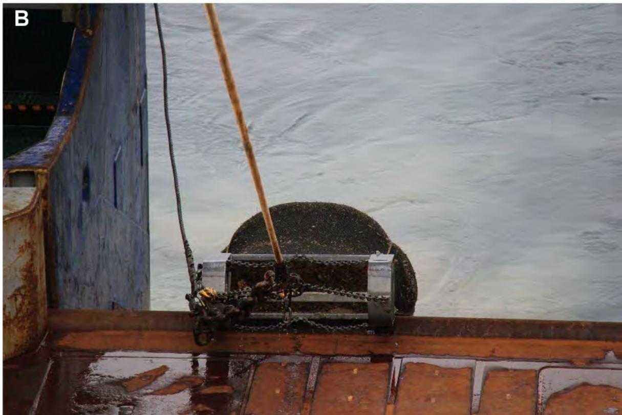
Figure 11: Agassiz Sled. A: on deck ready for deployment. B: being recovered up the stern ramp with a sample.
