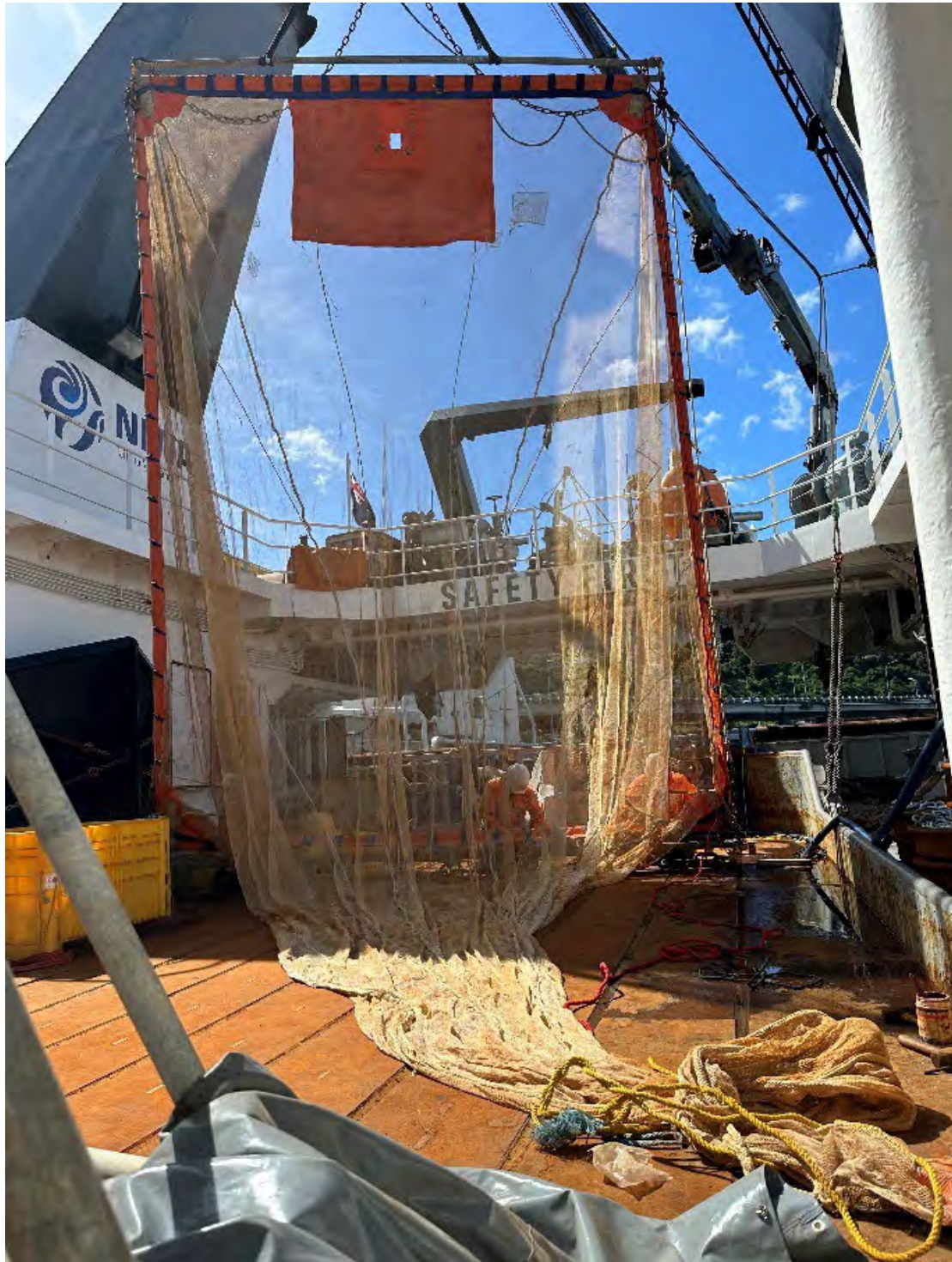
Figure 17: The rectangular mid-water trawl (RMT) vertically extended on deck during rigging. (Photo: Sadie Mills).
