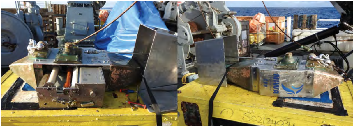
Figure 16: The Continuous Plankton Recorder including cassette (left) that is being loaded into the body (right).
