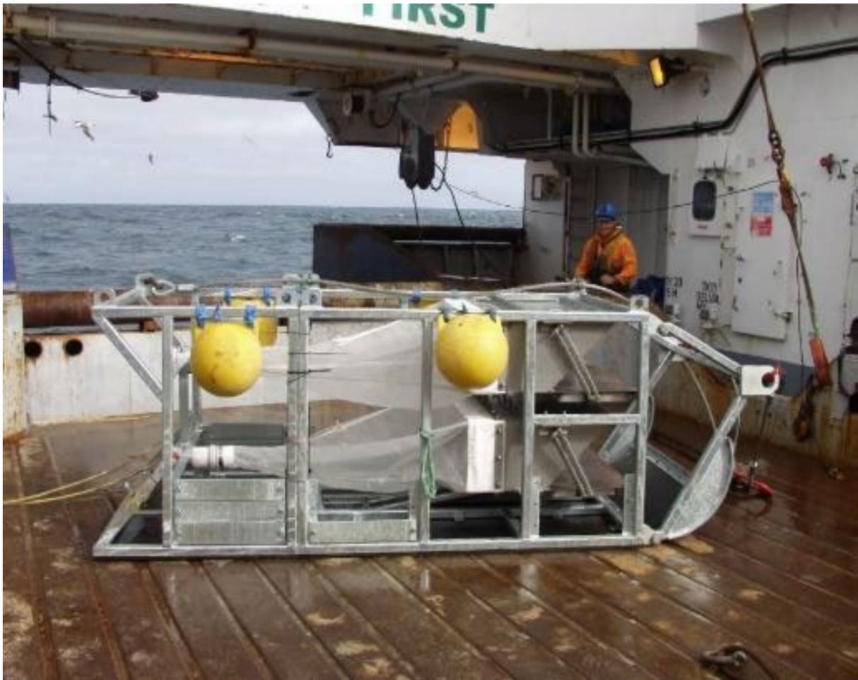
Figure 3-13: Hyperbenthic (Brenke) sled with 1500 m rated floats in towing position.
