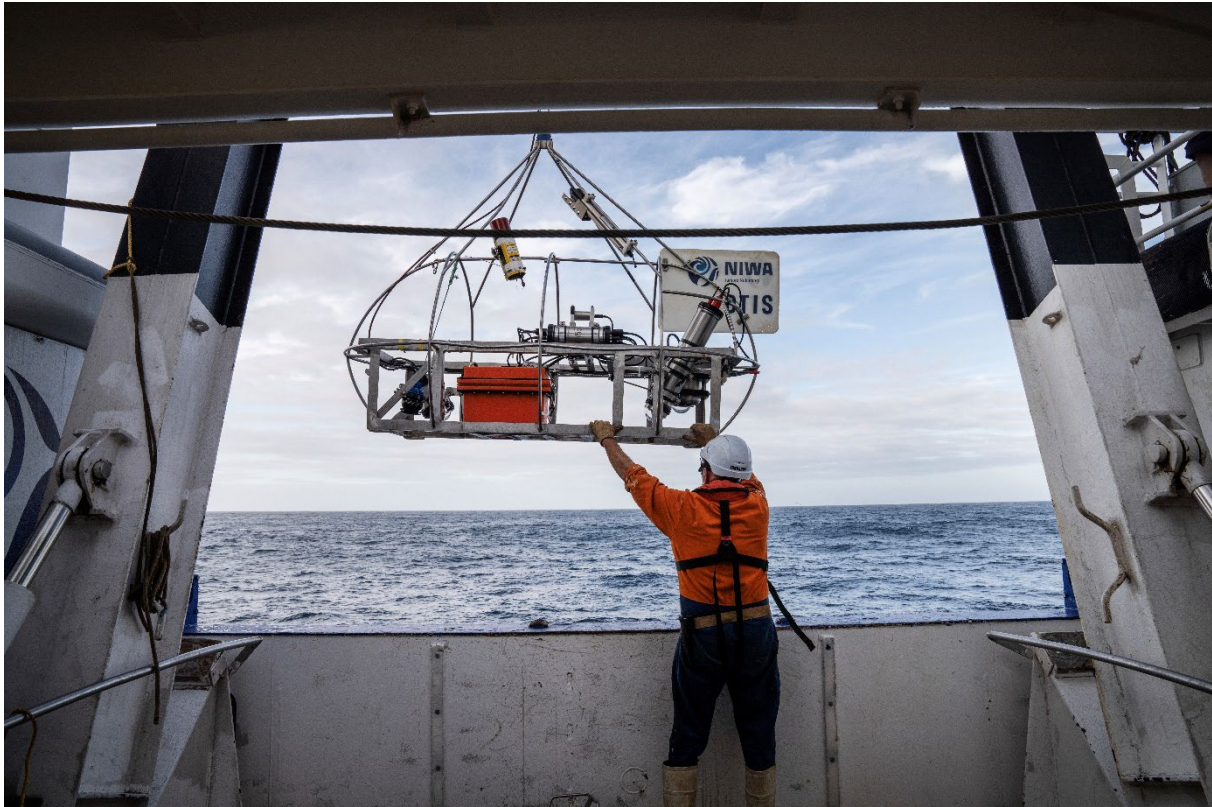
Figure 3-4: NIWA's Deep Towed Imaging System (DTIS). [Photo: Rebekah Parsons-King, NIWA].
