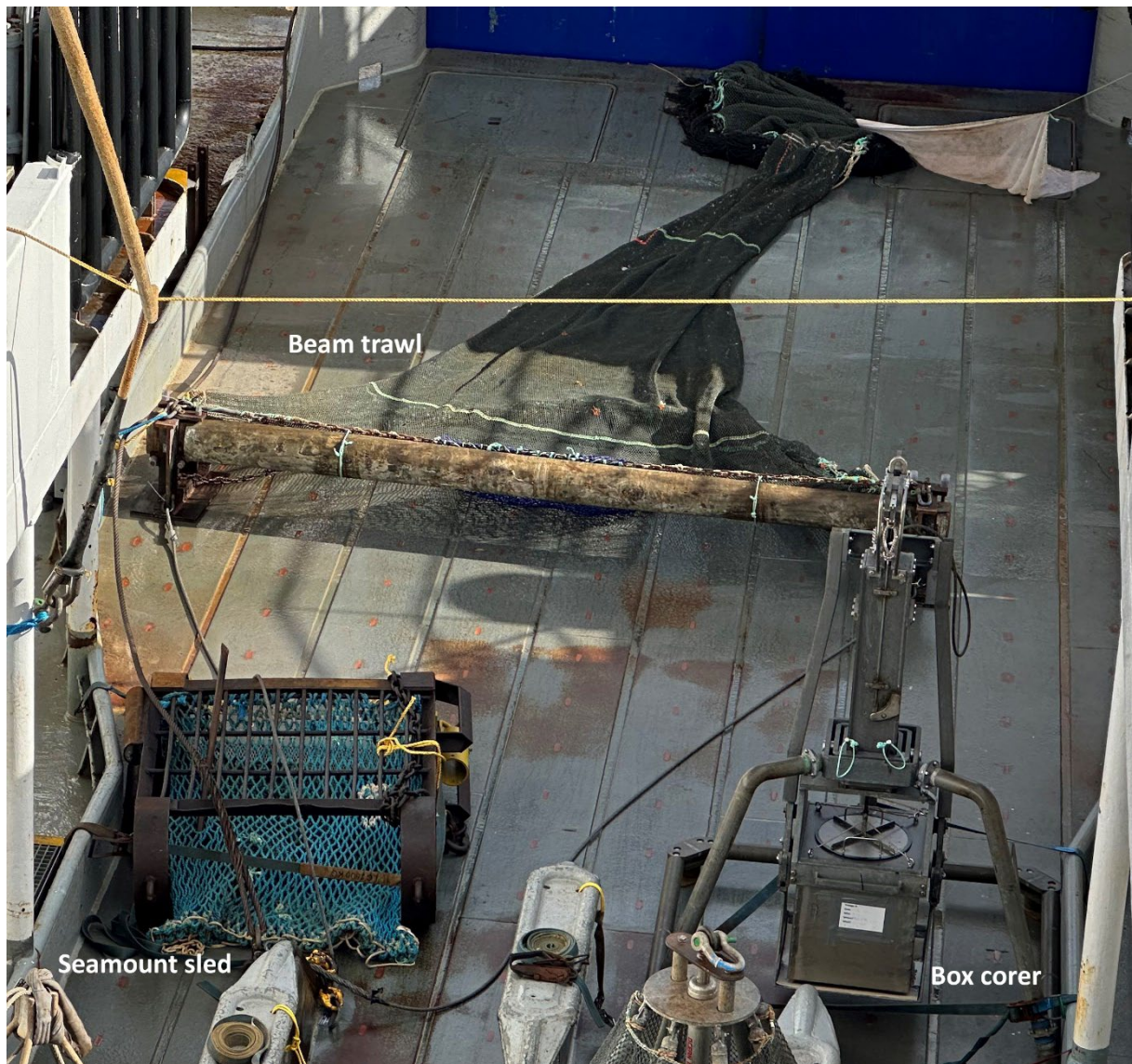
Figure 3-9: Seamount sled, designed to sample larger organisms living on the seabed on rocky, hard seafloor (lower left). Beam trawl designed to sample on soft flat terrain (top of image) [Photo: Sadie Mills]. Box corer is also depicted in the image (bottom right) but was not used during the survey.
