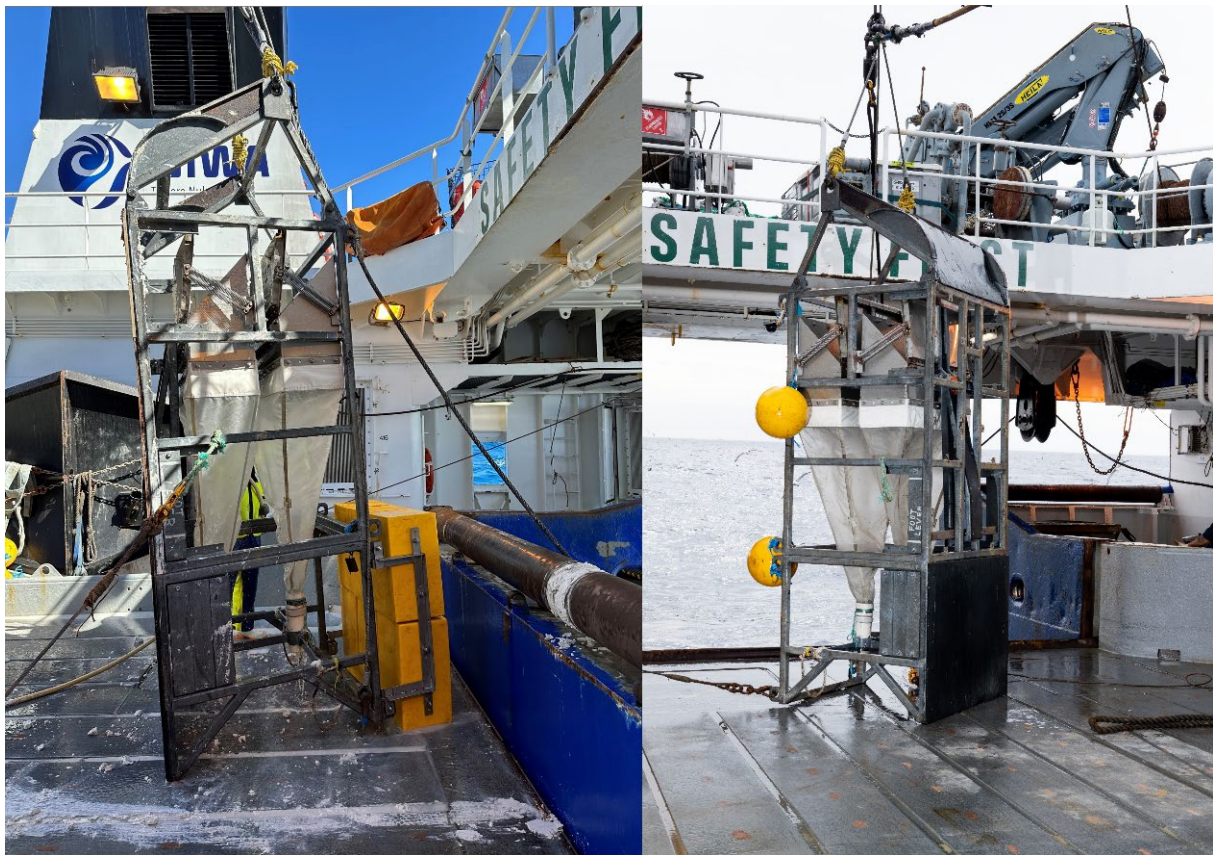
Figure 3-14: Brenke sled in upright position for retrieval of sample from cod ends, fitted with syntactic foam 6000 m rated floats (left) and 1500 m rated floats (right). [Photo: Sadie Mills & Rebekah Parsons-King, NIWA].
