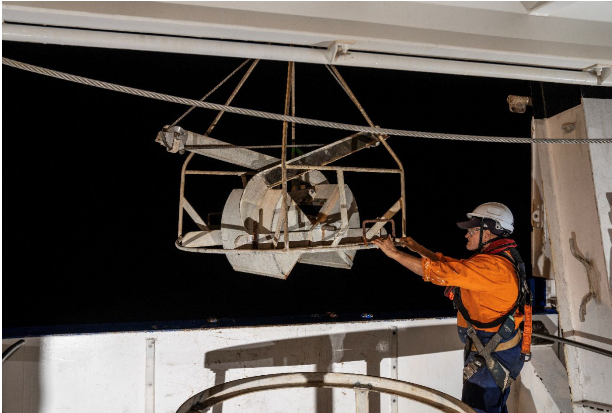
Figure 3-8: Van Veen Grab used for collection of faunal and sediment samples. [Photo: Rebekah Parsons-King, NIWA].
