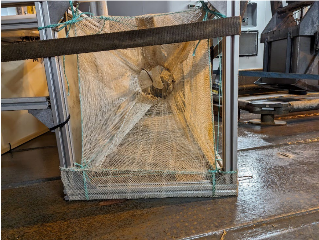
Figure 3-17: Redesigned funnel entrance using the finer mesh. [Photo: Thom Linley, Te Papa]
