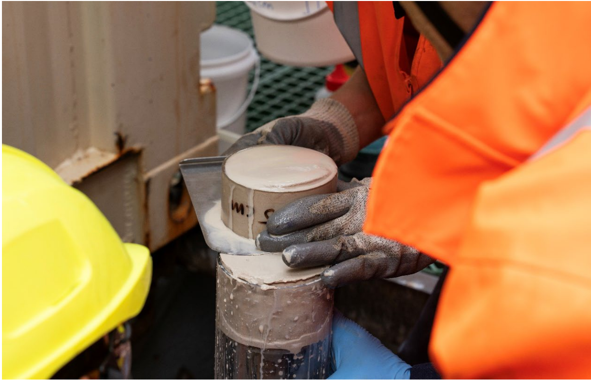
Figure 3-6: Sediment being sliced in 5 cm sections from an extruded multicore tube for macrofauna. [Photo: Rebekah Parsons-King, NIWA]
