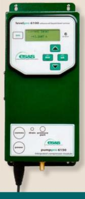
A 'bubbler' or 'gaspurge' water-level instrument, such as the Levelpro 6150 (pictured), is well suited to groundwater monitoring, as no sensitive equipment needs to be underwater. Just lower a simple plastic tube, through which compressed air is bubbled. The pressure on the gas from the weight of water is measured by a sensor above ground, and converted into a water level reading. [Photo: es&s]
