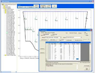
Example screen from TDGauge showing data from one location on the Selwyn River, Canterbury. Length and direction of vectors on the graph show the strength and relative direction of currents at gauged points. Here the gauging editor screen is being used to modify the selected gauging. Note the context sensitive help that explains what should be entered in the current field.
