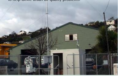
Together, we have been working to install five urban meteorological monitoring stations and link existing air quality monitors to them. Over time, the data from these stations will be used to create a baseline against which future air quality can be compared, as the councils implement air quality initiatives. The data will also be used to allow robust meteorological modelling to identify contributing sources of pollution.
