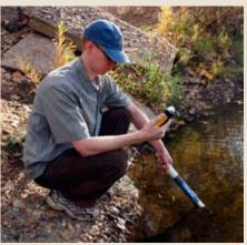
sensors in a hand-held wand, and a rugged pocket-sized display unit. Uses include: surface water-ground water interaction, stream restoration, wastewater effluent and stormwater runoff monitoring, dredging operations, low-flow sampling, and aquaculture. These sensors contain
