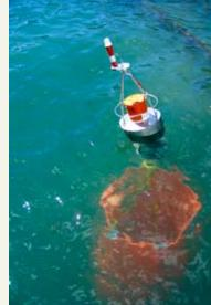
GPS drifter beside a mussel farm in the Marlborough Sounds. An underwater sail ensures the buoy moves with the currents not the wind. (Photo: Warren Thompson)
