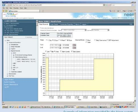
Example of information provided by the Neon system – the total volume (in cubic metres) of water supplied over a 36 hour period.
