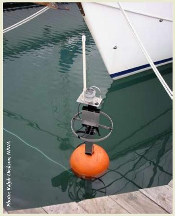
Our new salinity/turbidity buoy undergoing testing at the Nelson marina.
