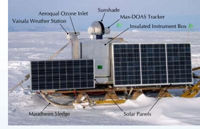
The prototype MAX-DOAS instrument built at NIWA Lauder. This year the team used a diesel generator to supplement the solar panels since the instrument must be kept running at all times to avoid freezing. Next year, they hope to add a small wind turbine instead. Logistical support by Antarctica New Zealand is gratefully acknowledged. [Photo: Tim Hay, NIWA/Canterbury University]
