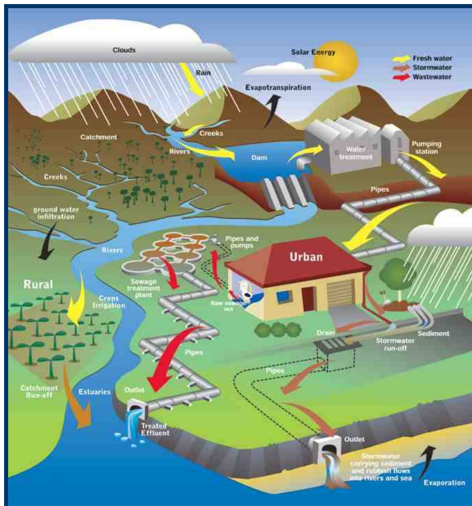
Figure 4: A more detailed description of the urban water cycle showing common urban infrastructure
