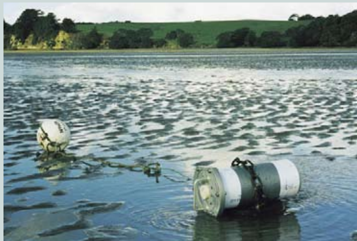
DOBIE moored in Okura Estuary (North Shore) for measuring waves on the intertidal flat.
