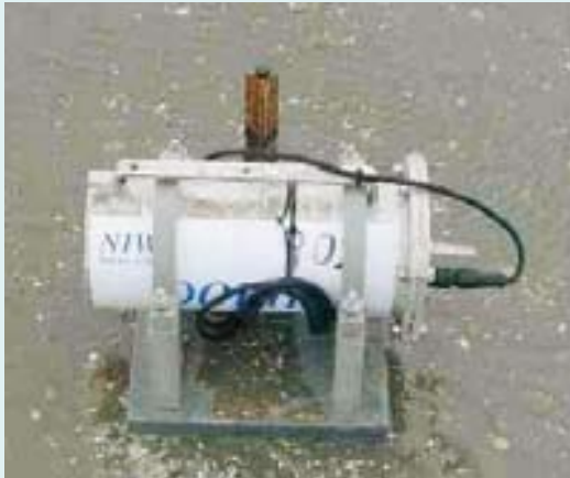
A DOBIE at one of the sandflat sites. DOBIE wave gauges measure water pressure, and from this calculate wave height, wave period and water depth. Some DOBIEs also measure the suspended sediment concentration of the water using an optical backscatter sensor (see Water & Atmosphere 11(1) : 11–13). (Photo: C. Lundquist)
