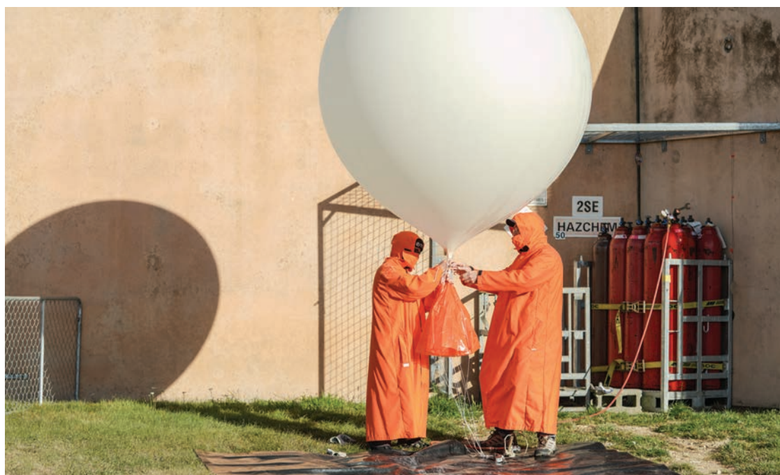
Researchers wearing fire protection coats release a hydrogen-filled weather balloon. Launched weekly, sensors tethered from the balloon gather valuable readings from the atmosphere more than 35km above. (Rebekah Parsons-King)
