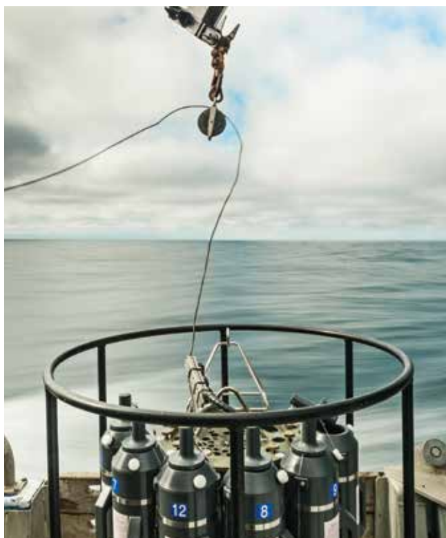
A vital part of the kit for measuring ocean acidification, the CTD (Conductivity, Temperature, Depth) profiler is lowered to different depths throughout the water column to capture samples and valuable data. (Dave Allen)
