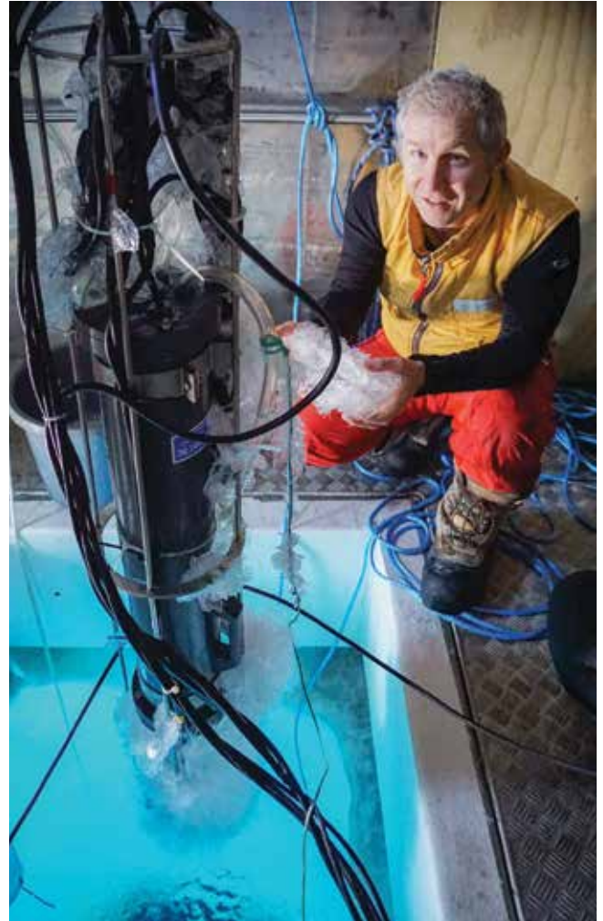
Craig Stevens removes ice crystals which have formed on the ‘supercoolometer’. (Brett Grant)
