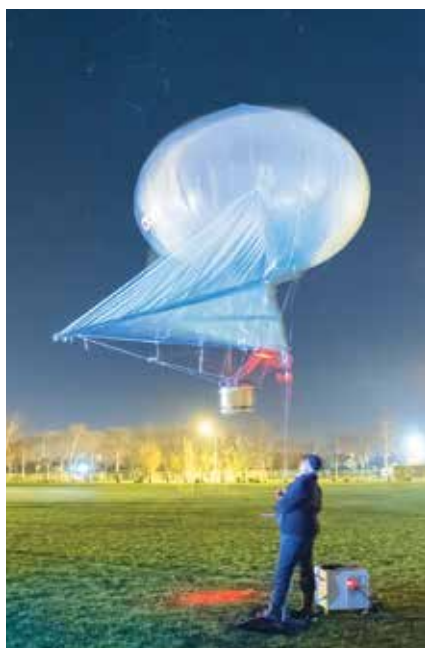
Environmental Monitoring Technician Sally Gray deploys a helium kite to observe layers of air pollutants in Rangiora. (Dave Allen)
