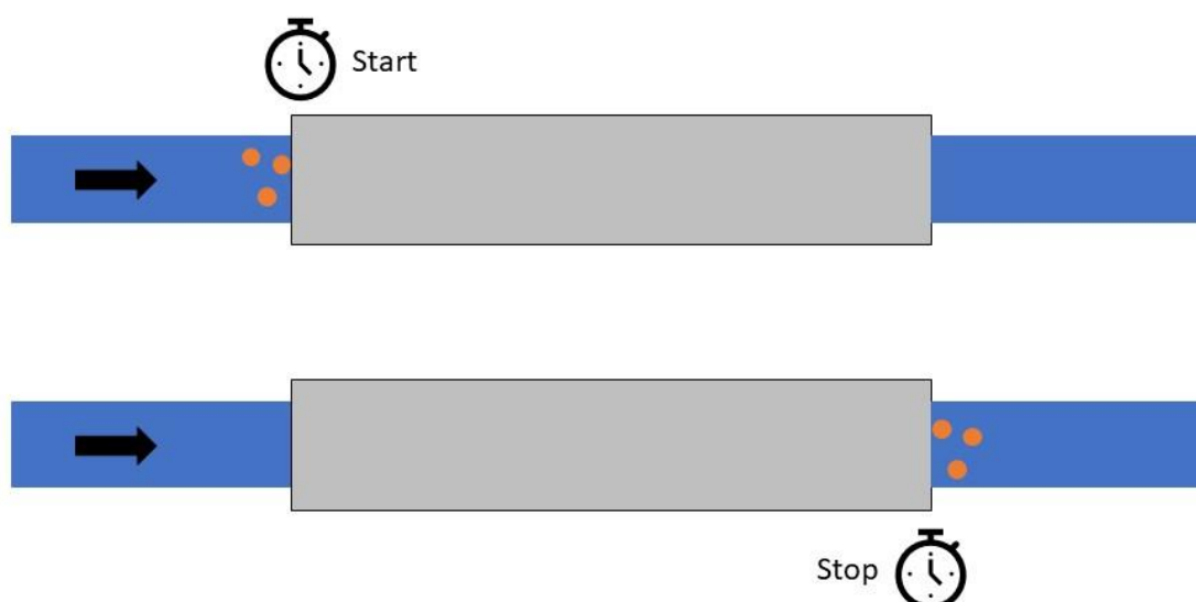
Figure C-2: Illustration of how to use the float method of measuring water velocity. The floats are released upstream of the culvert. A stopwatch is started as the floats enter the culvert. The time taken for each float to reach the other end of the culvert is recorded. This is used to calculate water velocity.
